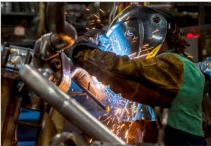
Travis Simmons of Grottoes welds pipe sections onto a catalytic converter at Walker Manufacturing in Harrisonburg on Oct. 20. (Photo by Daniel Lin / DN-R)
